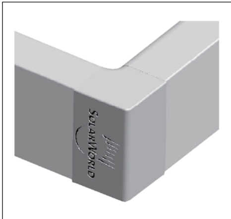
New corner connection Front view
